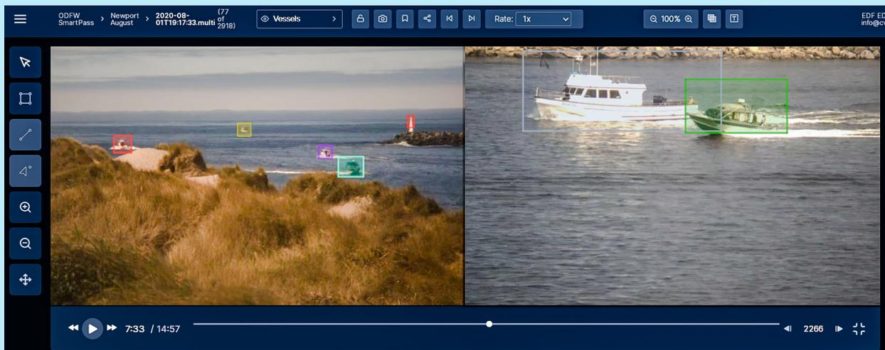
**Figure 6.** Snapshot of the review platform designed for the Oregon pilot. Shown here is the pass at Newport, OR with the bar view on the left and the cross-channel view on the right, and bounding boxes around the detected fishing vessels.
